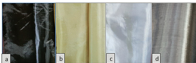
Figure 2 Fiber reinforced polymer fabrics: a) Basalt based FRP, b) Aramid based FRP, c) Glass based FRP, d) Carbon based FRP
