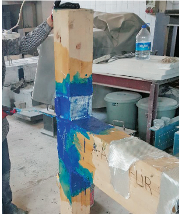
Figure 3 Strengthening stage with fiber reinforcement polymer fabrics Slika 3. Faza ojačanja polimernim tkaninama s dodanim vlaknima
