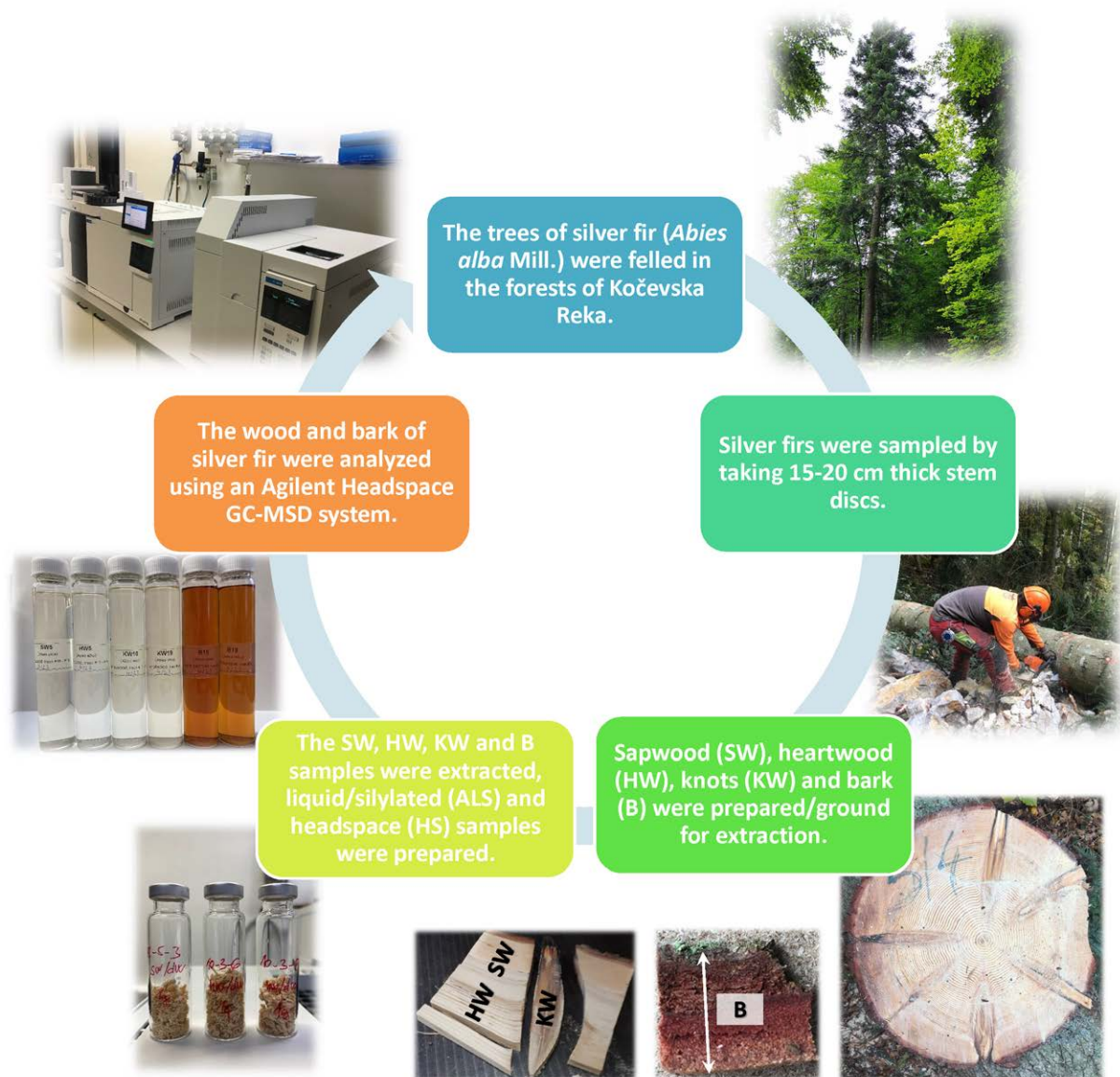
Figure 1 A scheme of analysis: Trees of silver fir ( Abies alba Mill.) were felled in the forests of Kočevska Reka, Ravne district. Sapwood (SW), heartwood (HW), knotwood (KW) and bark (B) of silver fir were prepared for extraction, the extracts were analyzed with a GC-MSD system equipped with automatic samplers for liquid samples and headspace samples. Slika 1. Shema analize: stabla jelovine ( Abies alba Mill.) posječena su u šumama Kočevske Reke, kotar Ravne. Bjelika (SW), srž (HW), kvrga (KW) i kora (B) jelovine pripremljeni su za ekstrakciju, a ekstrakti su analizirani sustavom GC-MSD opremljenim automatskim uzorkivačima za tekuću i hlapljivu fazu ekstraktivnih tvari.
