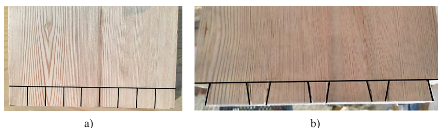
Figure 15 Marking patterns for making dovetail corner joints: a) straight teeth of a dovetail joint, b) angled teeth of a dovetail joint
