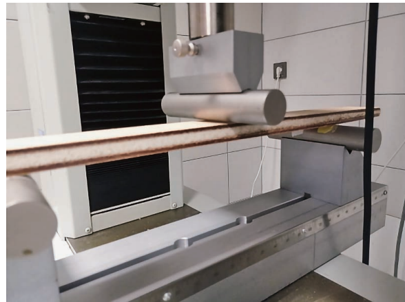
Figure 1 Bending test of sandwich panels constructed in the study
