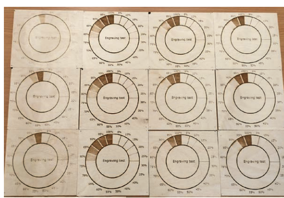
Figure 6 Results of an engraving test and changes in discoloration of birch plywood at \Delta F = -8 mm
