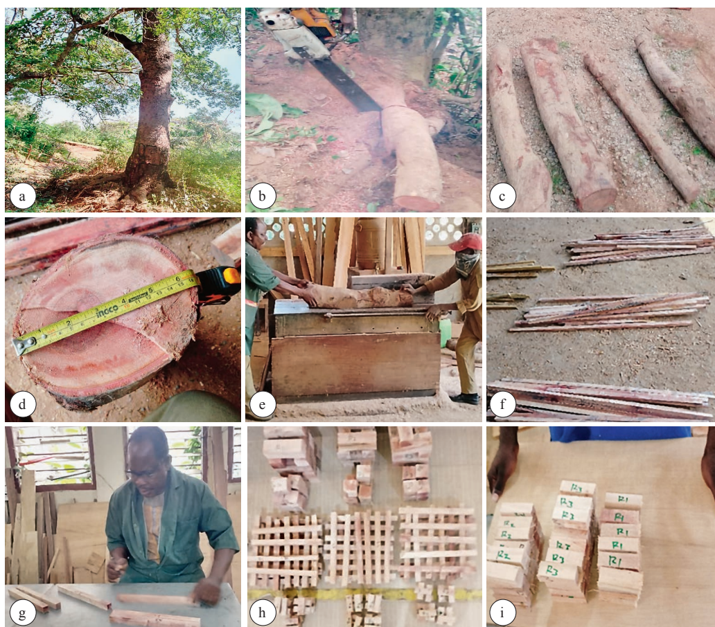
Figure 1 Root wood samples preparation for physical and mechanical tests
