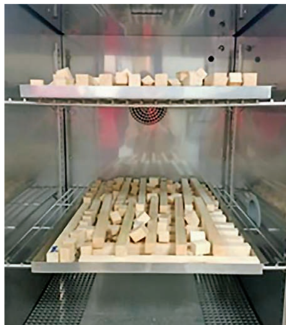
Figure 2 Conditioning of the prepared test samples in the climate chamber
