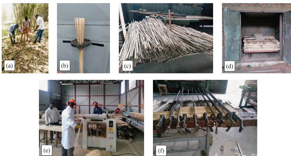
Figure 1 LBL manufacturing process: Bamboo culm harvesting and sectioning (a), culm splitting (b), split strips (c), kiln drying strips (d), planing strips (e), and clumping strips which is glued with UF resin (f)
