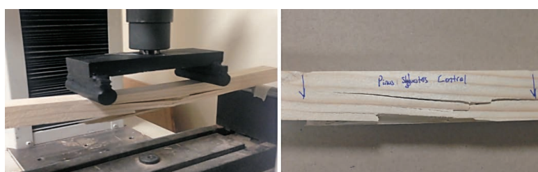
Figure 3 Type of fracture observed in wood material
