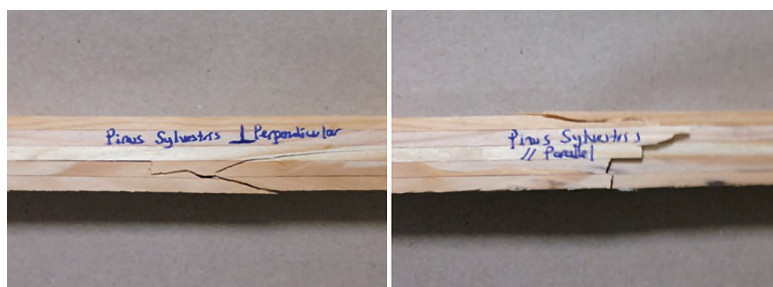
Figure 4 Type of fracture observed in laminated wood material
