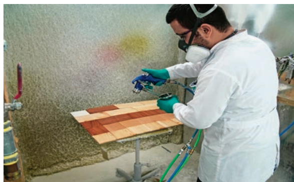
Figure 2 Images of the application process of daylight UV-curable and high-energy UV-curable varnishes Slika 2. Prikaz postupka nanošenja UV lakova
