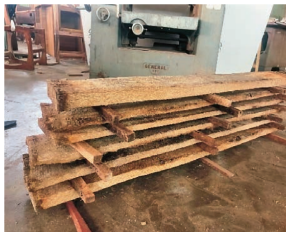
Figure 19 Seasoning of coconut timber Slika 19. Sušenje drva kokosove palme
