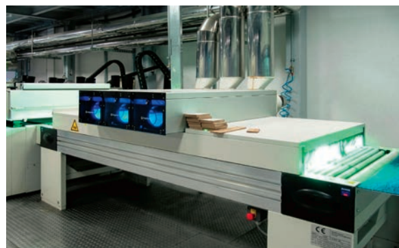
Figure 2 Images of the application process of daylight UV-curable and high-energy UV-curable varnishes
