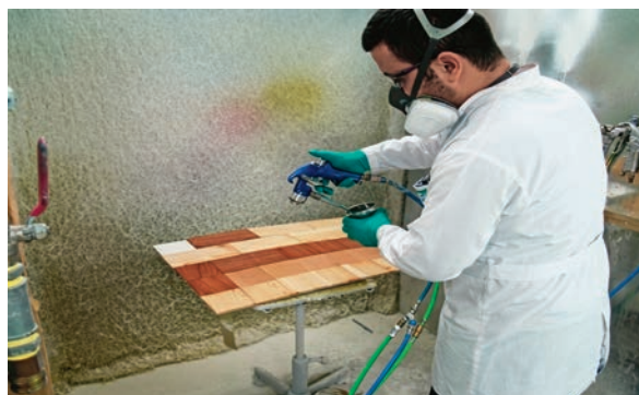
Figure 2 Images of the application process of daylight UV-curable and high-energy UV-curable varnishes
