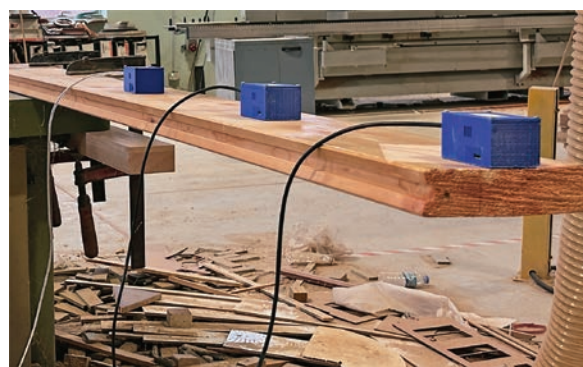
Figure 10 Some images of cantilever vibration measurement setup
