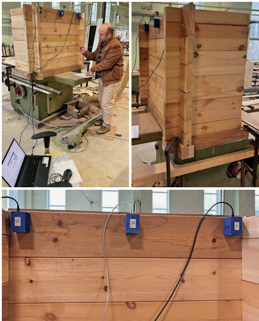
Figure 11 Sample images of individual element vibration measurement setup
