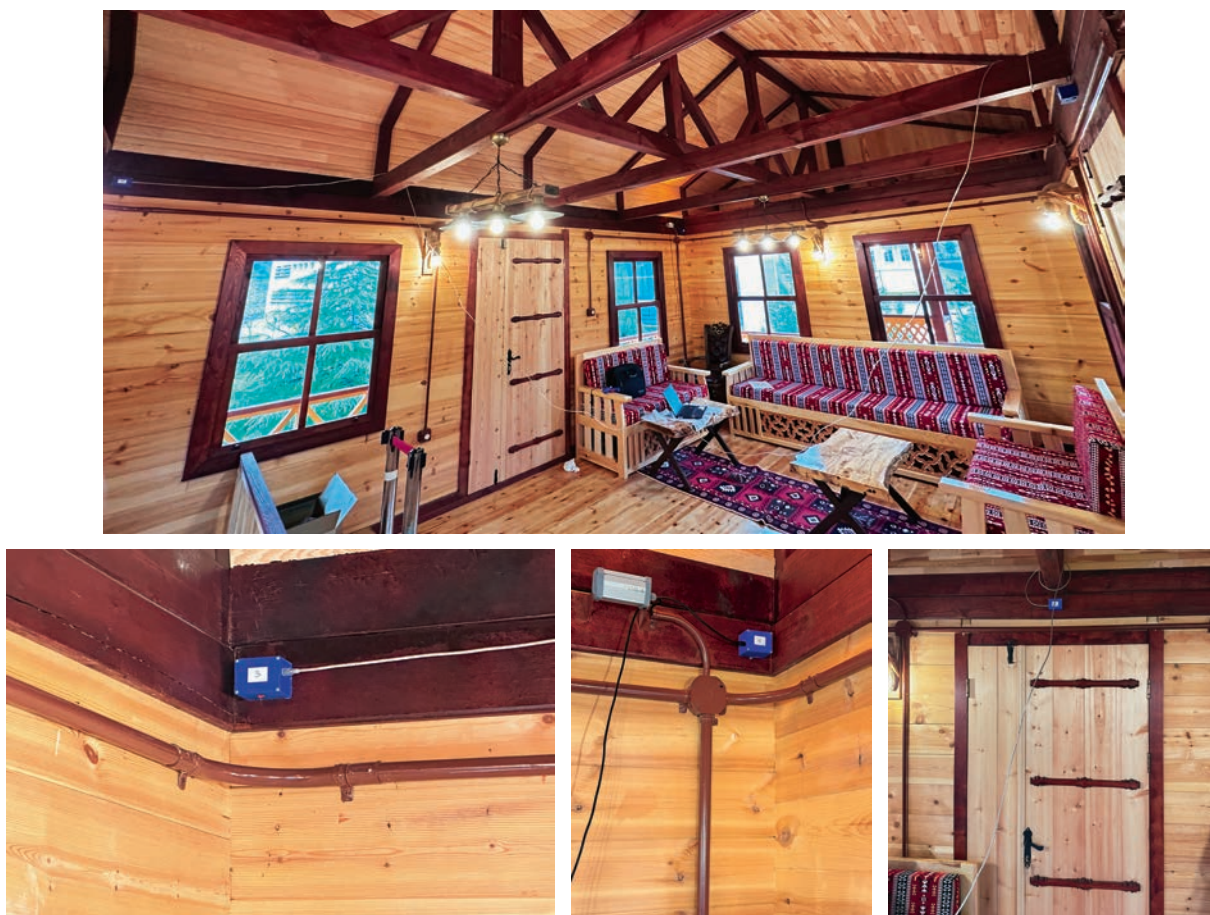
Figure 5 Sample images of vibration measurement setups (CEVS)
